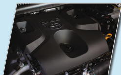
1GD-FTV Engine with 6 Speed MT Transmission
