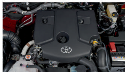
2.8L 16D ENGINE WITH 201 HP MAX OUTPUT & 500 NM MAX TORQUE
