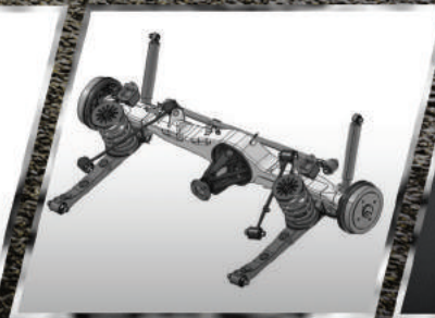
4-link with Lateral Control Rod rear suspension
